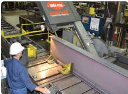
State of the art sawing systems deliver accurate miter saw cut parts.
